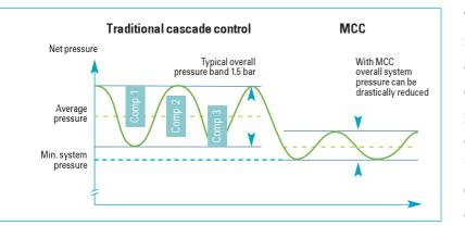
The Elektronikon® MCC offers a significant opportunity to reduce the overall system pressure band in comparison with traditional cascaded compressor control. Every 1 bar reduction of the average system pressure stands for 7% energy savings. Losses of compressed air due to system leakage are reduced with 13%. These two factors can account for overall energy savings of 10% over the lifetime of your compressors.
